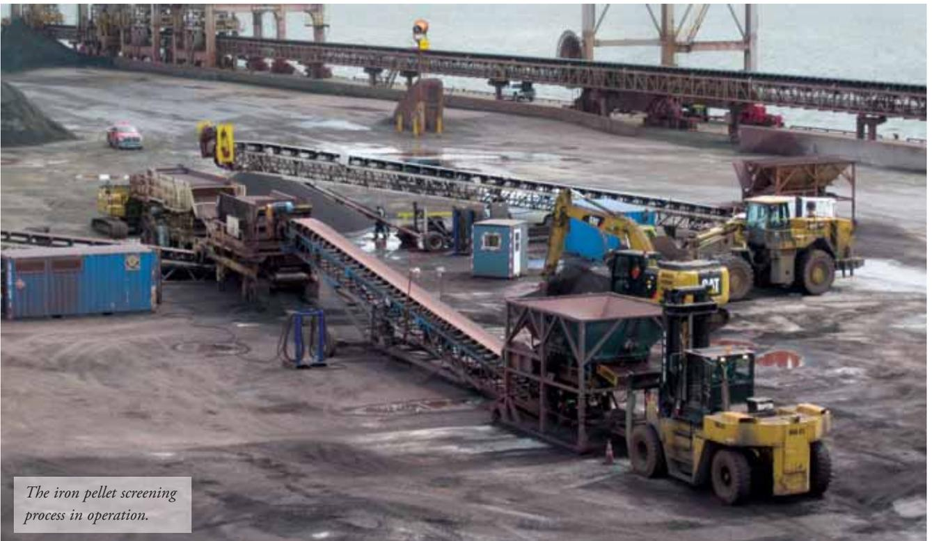
*The iron pellet screening process in operation.*
